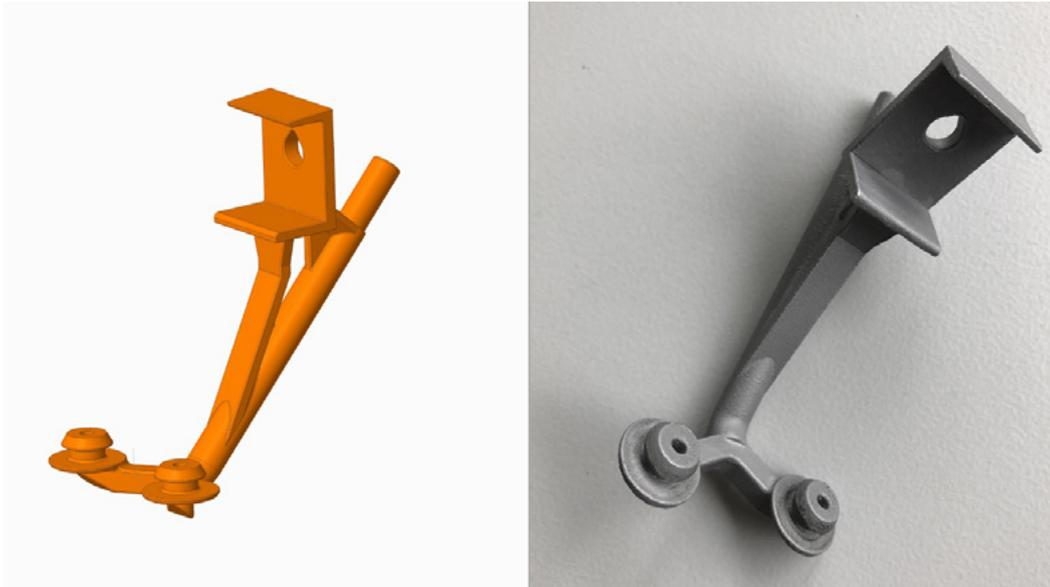
*The suction pipe (on the left as a model, on the right the final product) with its hollow space and complex shape is virtually predestined for 3D printing. This part is built into the ProLiner in small numbers, which is why it is produced in series using a metal 3D printer.*
