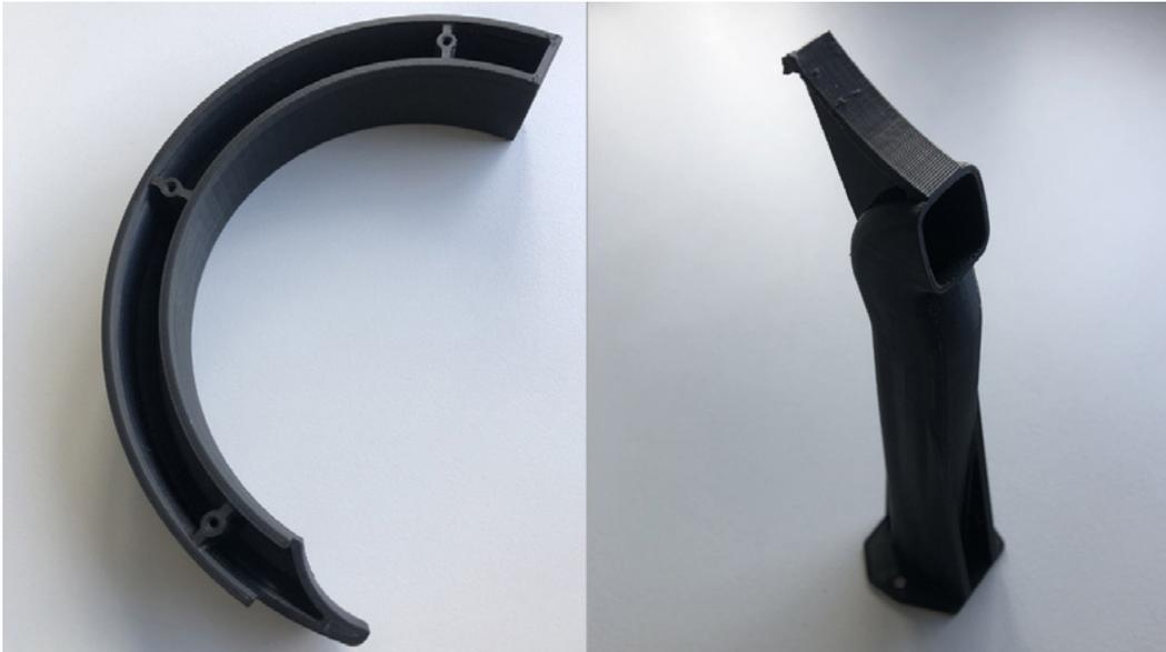
*The supporting stand (left) and the blow air finger are classic examples of how 3D printing is being used at Muller Martini. The prototypes were produced using 3D printing, while the series parts are manufactured using plastic injection molding. They are used in saddle stitchers.*
