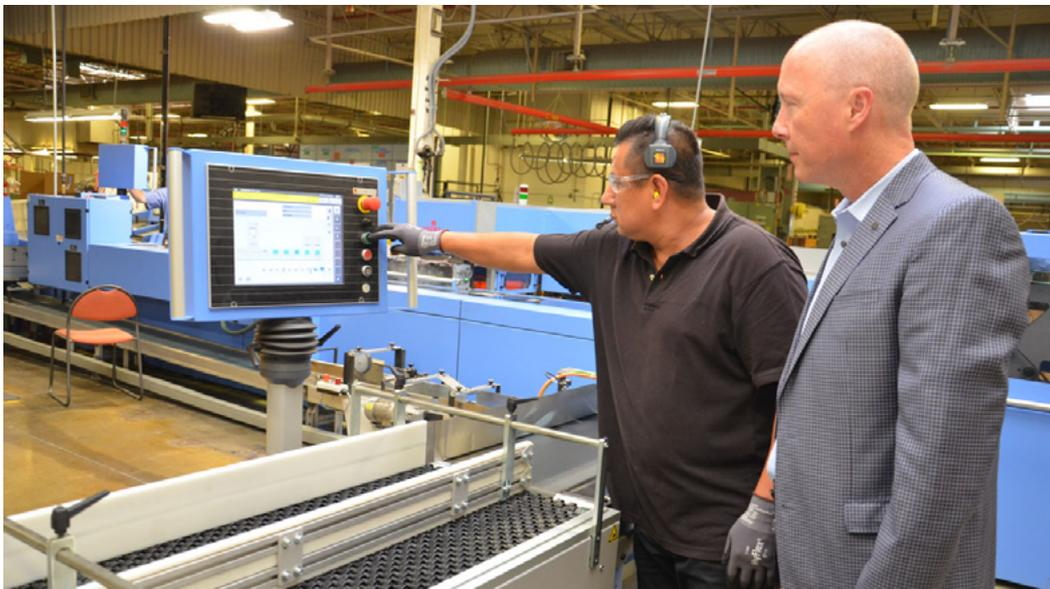
Israel Bonfil (machine operator at Core Publishing Solutions) together with Eric Olsen (Sales Manager at Muller Martini North America) at the signature stack feeder for digitally printed products, which is located as a special configuration between the gathering machine and the Alegro Digital binder in Eagan.
